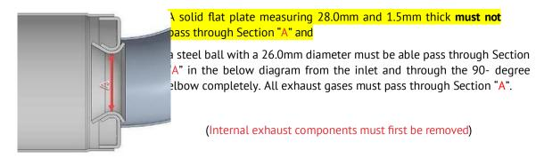
The inner measurement of the exhaust system silencer end (a) in the diagram must be a maximum of 63.0 mm.
