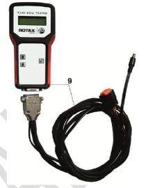
Connect energy cable of ECU tester cable harness with the charging connector of engine cable harness.
