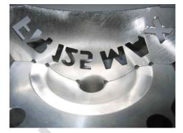
Casted wording "ROTAX" and/or "MADE IN AUSTRIA" must be shown.
