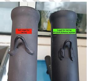
**5.14.2 125 Micro MAX (Micro Cadet) Perforated Tube & Isolation Mat** Perforated tube ROTAX part number: 273212.
